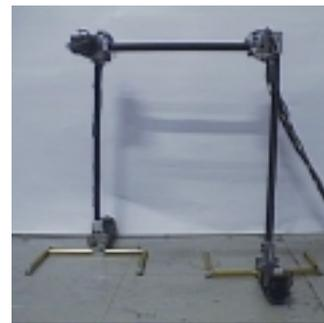
Fig.3 4 joint 3 link biped robot
