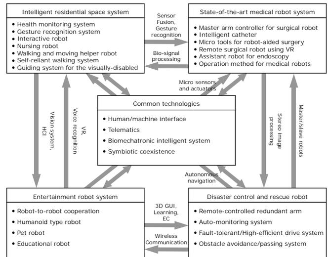
Fig.5 Related technologies for human-friendly welfare robot systems
