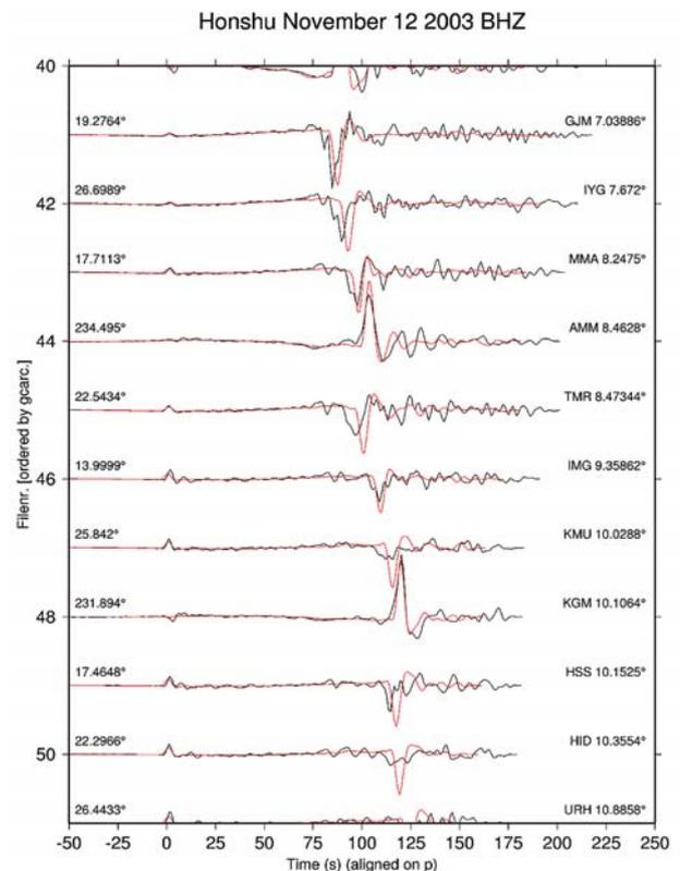
Fig. 1 Broadband data and synthetic displacement seismograms for the 2003 South of Honshu earthquake bandpass-filtered with a two-pass four-pole Butterworth filter between periods of 3.5 and 150 seconds. Vertical component data (black) and synthetic (red) displacement seismograms aligned on the arrival time of the P wave are shown. For each set of seismograms the azimuth is printed above the records to the left, and the station name and epicentral distance are printed to the right.
