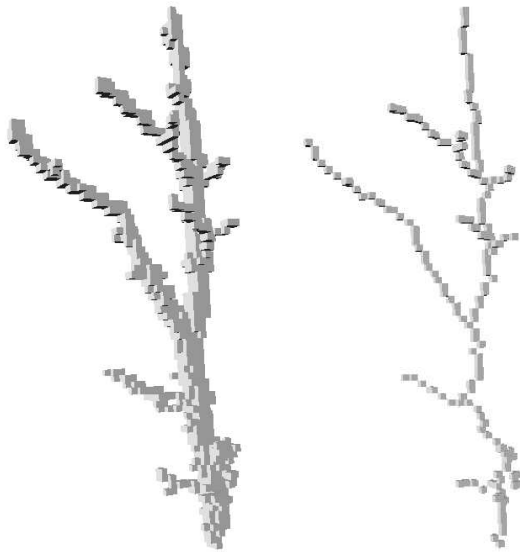
Figure 5: Skeletonization. Left: rasterized points; right: skeleton
