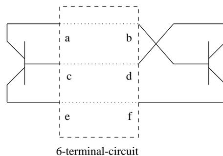
Fig. 1. Feedback structure consisting of two bipolar transistors. The remaining of the circuit is represented as a black box. The type of the transistors (n type or p type) is irrelevant.
