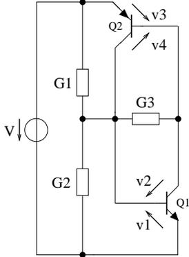
Fig. 2. S-type NDR circuit: if present, the feedback structure causes the circuit to exhibit NDR if values of conductances are appropriately chosen. Any two of the three resistors may be open-circuited. The NDR disappears if all three resistors are open-circuited, even though the feedback structure exists.
