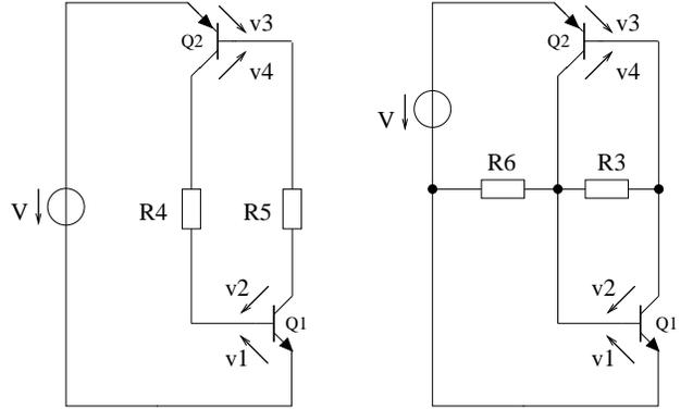
Fig. 3. The coefficient criteria *may fail* to predict the presence of a feedback structure (left), or it *may successfully* do so (right).
