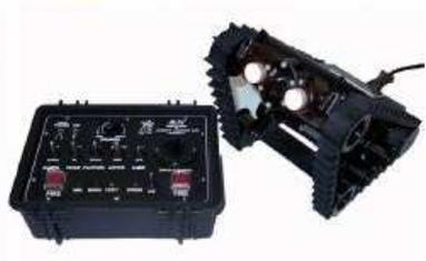
Fig. 1. A Field X man-packable inspection robot.
