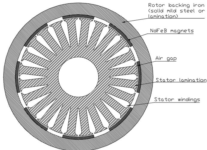
Figure 1. Cross-sections of the surface-mounted PM generator.
