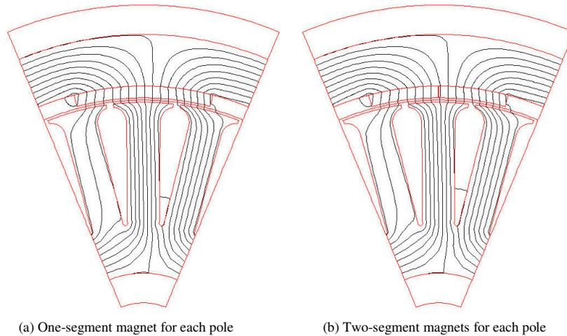
Figure 4. Flux plot of the generator when rotor is at 360 ° (electrical).
