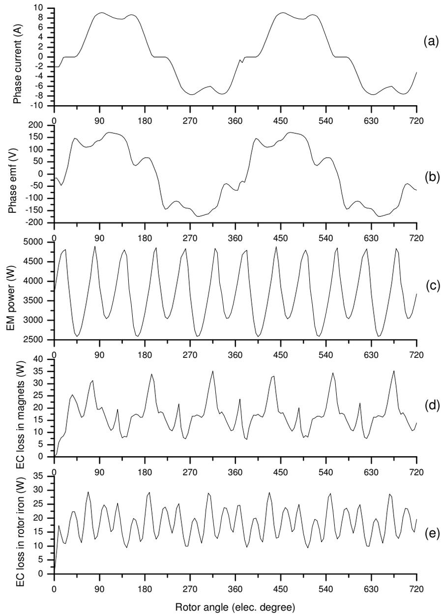
Figure 3. Stator phase current (A), stator phase emf (V), electromagnetic power (W), eddy-current losses (W) in the magnets and rotor backing-iron, for a PM generator with 4 mm thick magnets and 1.5 mm air gap, rotating at 3000 rpm.
