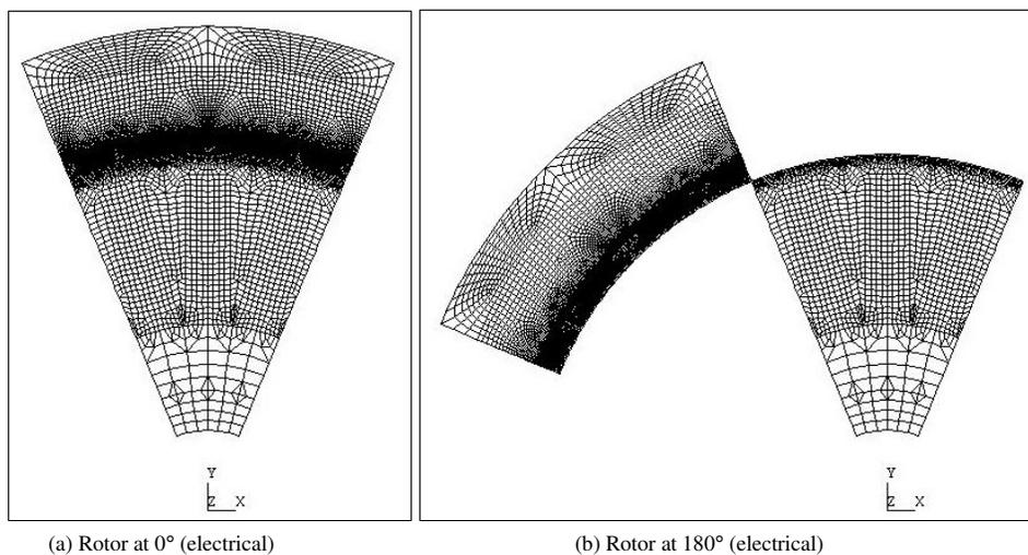
Figure 2. Finite element meshes.
