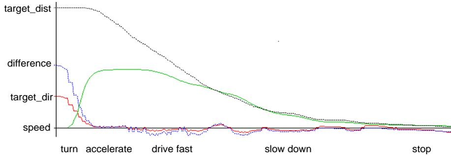
**Fig. 3.** Recording of two sensors (distance and direction of the target) and two actuators (average motor speed and difference between the two motors) during a simple taxis behavior. The robot first turns towards the target, then accelerates, drives fast, slows down, and finally stops at the target position.
