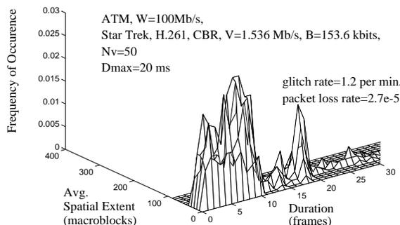
Figure 8: Histogram of the glitch duration and spatial extent for an ATM multiplexer, Star Trek sequence, H.261, CBR,  $D_{max}=20$  ms.
