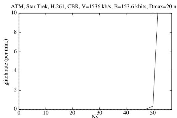
Figure 7: Glitch rate as a function of  $N_v$  for ATM, Star Trek VI, H.261, CBR,  $D_{\text{max}}=20$  ms.
