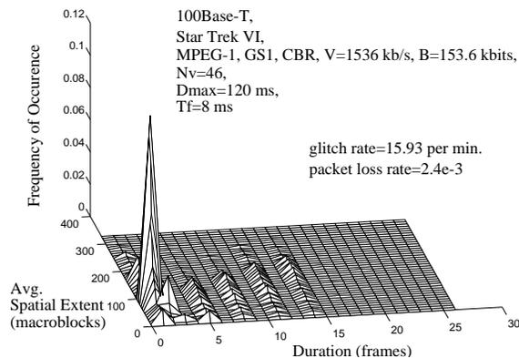
Figure 5: Histogram of the glitch duration and spatial extent for a 100Base-T Segment, Star Trek sequence, MPEG-1, GS1, CBR,  $D_{\text{max}}=120$  ms.
