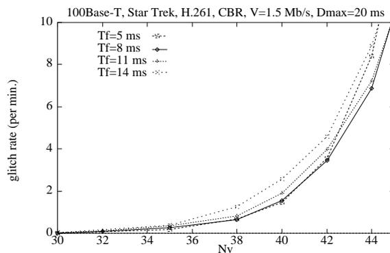
Figure 1: Glitch rate as a function of the number of video streams in a 100Base-T Segment, Star Trek sequence, H.261, CBR,  $D_{max}=20$  ms.
