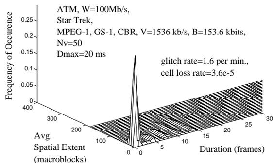
Figure 9: Histogram of the glitch duration and spatial extent for an ATM multiplexer, Star Trek sequence, MPEG-1, GS1, CBR,  $D_{max}=20$  ms.
