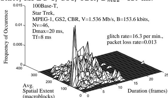
Figure 6: Histogram of the glitch duration and spatial extent for a 100Base-T Segment, Star Trek sequence, MPEG-1, GS2, CBR,  $D_{\text{max}}=20$  ms.
