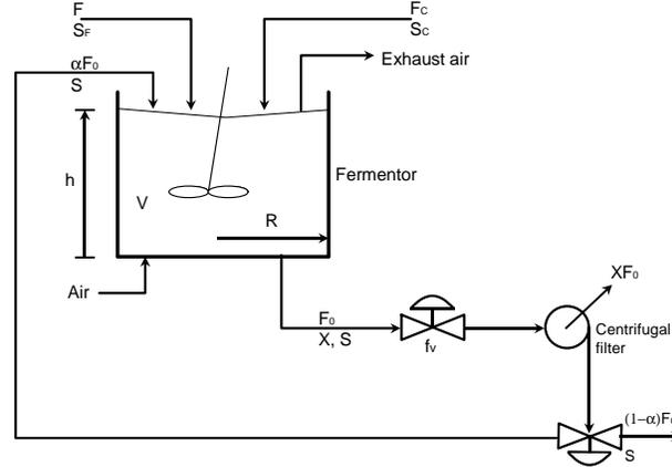
Figure 1. Flowsheet of the fermentation process. Reprinted from Brengel and Seider (1992).
