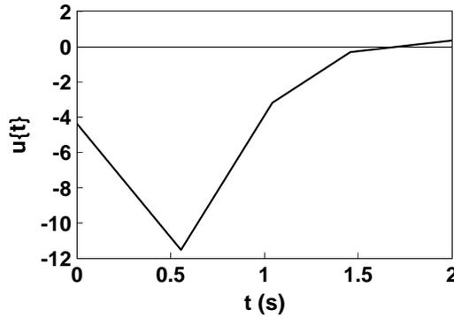
Figure 5. Optimal control for case study IV. The associated performance index is  $J=58.13$ .
