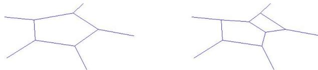
**Figure 4.2:**  $T_2^2$ -operation. On left a face of a simplex mesh before the operation is depicted. On right two new faces of a simplex mesh resulting from the operation are shown.
