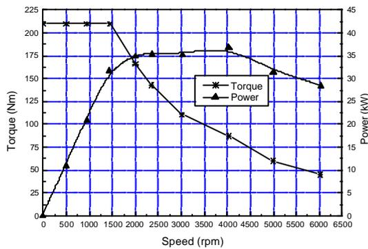
Fig. 5. Maximum torque and power for the prototype SRM
