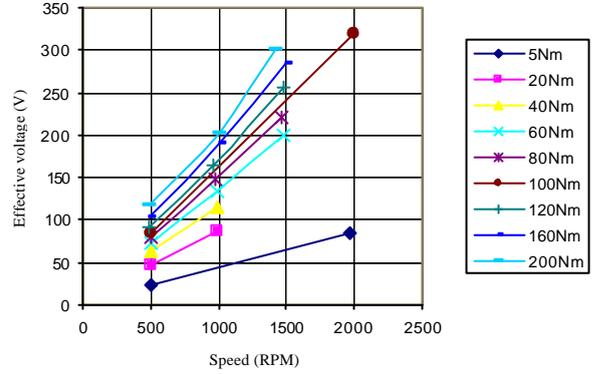
Fig. 12. Effective voltage for C2 ( $\theta_{on} = 180^\circ$ ,  $\theta_{off} = 30^\circ$ )
