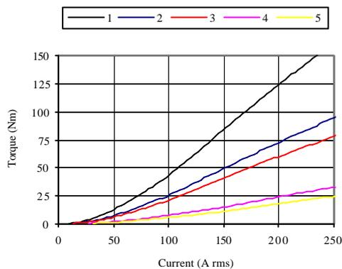
Fig. 14. FEA calculated torque versus current for C1
