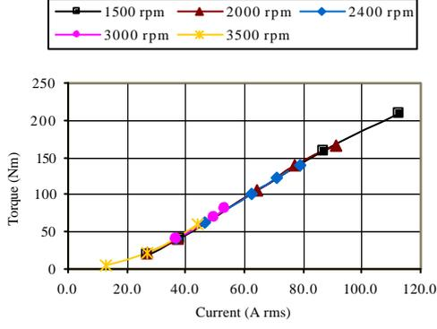
Fig. 8. Torque for commutation C3 ( $\theta_{on} = 210^\circ$ ,  $\theta_{off} = 60^\circ$ )
