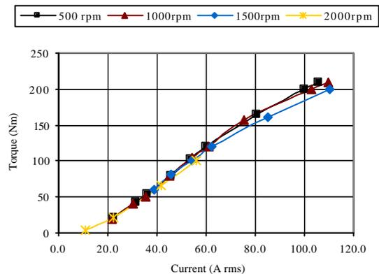
Fig. 7. Torque for commutation C2 ( $\theta_{on} = 180^\circ$ ,  $\theta_{off} = 30^\circ$ )
