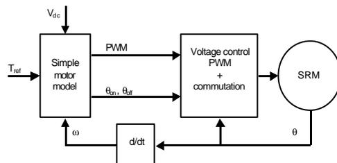
Fig. 4. Voltage controller
