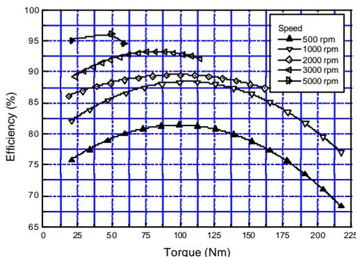
Fig. 6. Motor efficiency for the prototype SRM
