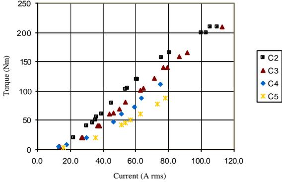
Fig. 11. Torque curves for commutation settings C2, C3, C4, C5
