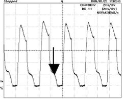
Fig. 10. Phase current (2000 rpm, 100 Nm)
