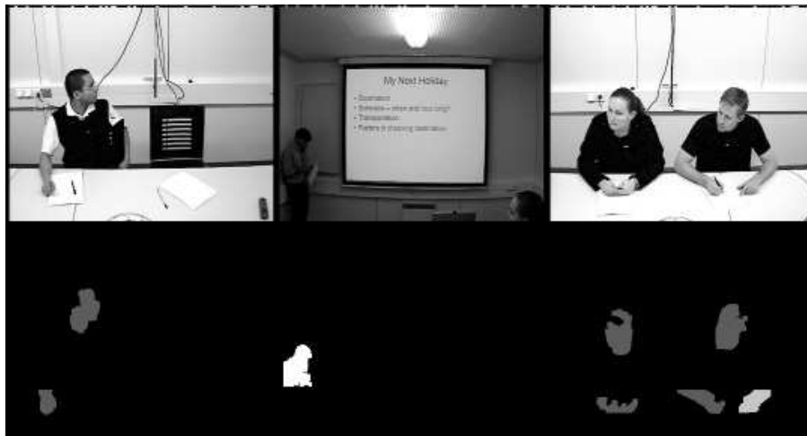
Fig. 3. Blob extraction in the multicamera meeting room. The top row of images shows a frame from each of the 3 cameras, and the bottom row shows the detected skin blobs (left and right) and moving blobs (centre).
