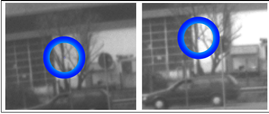
Figure 3. Wrong match due to different viewing angles eliminated by the trifocal tensor test.
