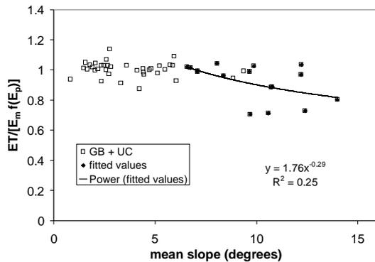
**Figure 2.** Influence of catchment mean slope on ET. Solid diamonds (overlaid on open squares) are the data values used in deriving the fit shown and comprise catchments in the Goulburn-Broken basin with high catchment mean slope. Open squares are the catchments used in deriving the influence of PE on ET.
