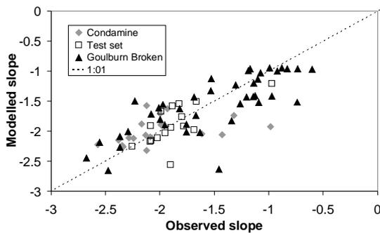
**Figure 4.** Modelled slope of flow duration curve against observed slope. Fit based on 40 catchments in the Goulburn-Broken basin.
