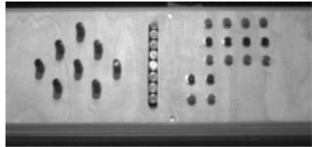
Figure 4. Button and knob layout on the box of the STRIMIDILATOR. On the left are the knobs, the lowest two are for the note-on and note-off velocity. In the middle are the switch buttons for the various modes. On the right are the note-on/off buttons.
