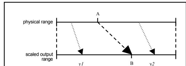
Figure 5. Dynamical mapping. When switching from one mode to another the last value (B) of the controller is put into memory and the next time the mode is entered, the controller value takes this value as a starting point; the physical value A is mapped to B. While the instrument is in this mode, all other values are mapped accordingly. For example, value  $x1$  is mapped to  $y1$  and  $x2$  is mapped to  $y2$ .
