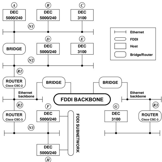
Figure 8: The subset of the Stanford Network used in the measurements
