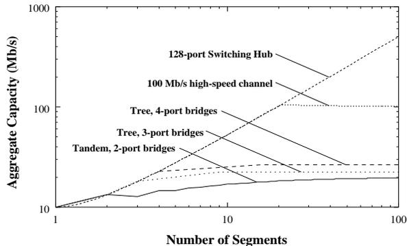
Figure 2: Aggregate throughput for the various subnetwork topologies
