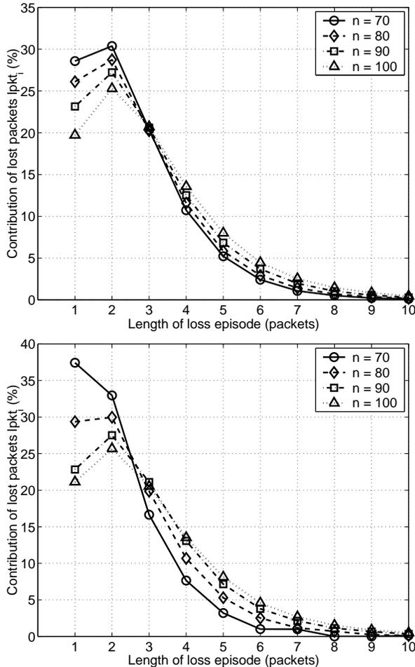
Figure 4: *Star Wars* trace, the number of sources =  $n$ , the buffer size  $B = 50$  kB (top) and  $B = 100$  kB (bottom). Contribution of lost packets from loss episodes of various lengths to the overall number of loss episodes.
