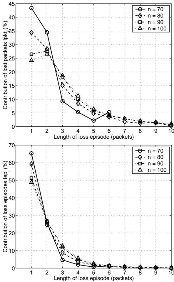
Figure 6: *Talk show* trace, the number of sources =  $n$ , the buffer size  $B = 100$  kB. Contribution of lost packets (top) and loss episodes (bottom) of various lengths to the overall number of loss episodes.
