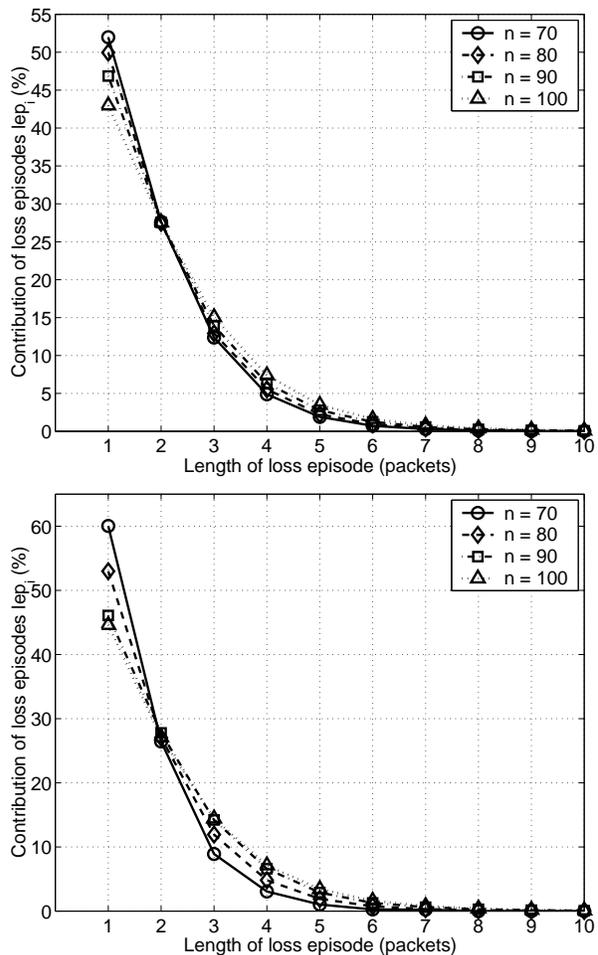
Figure 5: *Star Wars* trace, the number of sources =  $n$ , the buffer size  $B = 50$  kB (top) and  $B = 100$  kB (bottom). Contribution of loss episodes of various lengths to the overall number of loss episodes.
