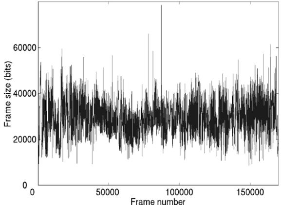
Figure 2: Traffic pattern of video trace (time scale = 1/24 sec). Frame sizes (in bits) are shown for more than 170,000 video frames. This corresponds to approximately two hours of an MPEG-1 video trace.
