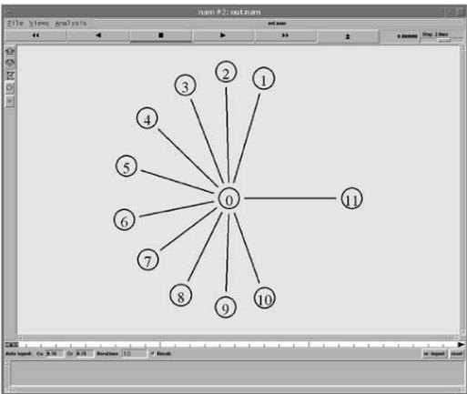
Figure 1: Screen dump from network animator *nam* for topology with  $n = 10$  sources. The topology is generated automatically. Node 0 is the router, nodes 1 to 10 correspond to the traffic sources, and node 11 is the traffic sink. The sources generate UDP traffic according to a supplied trace.
