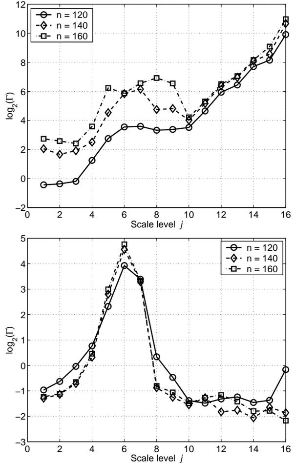
Figure 10:  $\log_2(\Gamma)$  vs.  $j$  plot of packet loss process for buffer size  $B = 69$  kB. UDP transfers (top) and TCP transfers (bottom)
