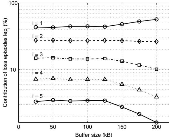
Figure 8: Percentage of loss episodes of length  $i$  ranging from 1 to 5 packets vs. the buffer size. *Star Wars* trace, the number of sources  $n = 100$ .
