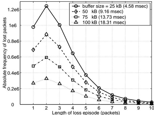
Figure 7: Total number of lost packets from loss episodes of length  $i$  packets. *Star Wars* trace, the number of sources  $n = 100$ . For better clarity of the figure, only the results for buffer sizes 25, 50, 75, and 100 kB are shown.
