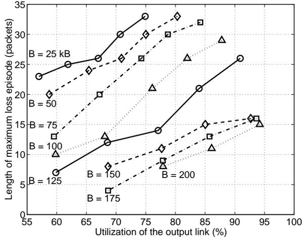
Figure 9: Length of the maximum loss episode vs. the utilization of the output link. The buffer is a parameter and ranges from 25 kB (4.58 msec) to 200 kB (36.62 msec).
