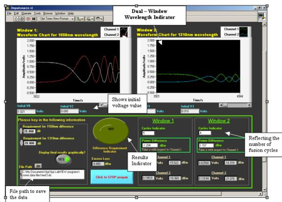
Fig. 6. GUI of the developed fibre fusion coupling workstation.
