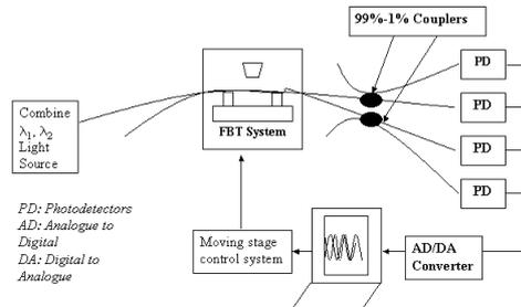
Fig. 4. Schematic illustration of the dual wavelength FBT system.
