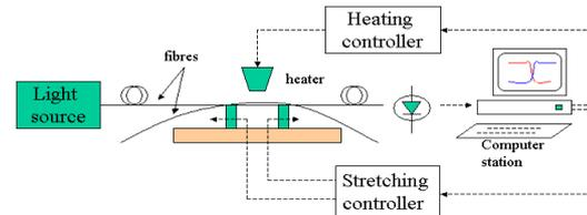
Fig. 1. Schematic illustration of fusing fibre couplers by the FBT technology.
