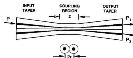
Fig. 2. Schematic diagram of a fused fibre coupler.
