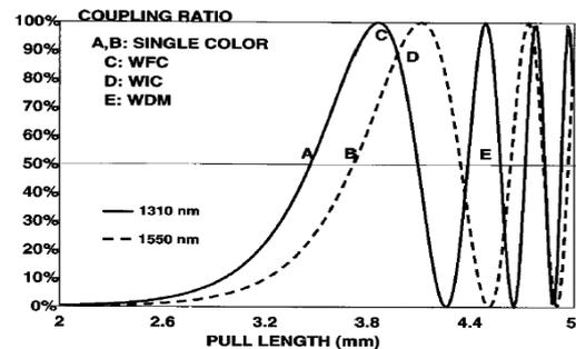
Fig. 3. Coupling ratio as a function of pull length for a fused biconical taper (FBT) coupler.
