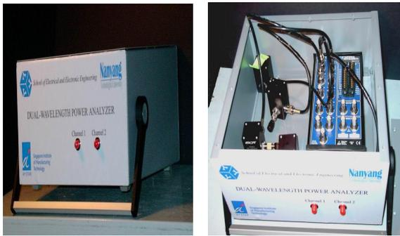
Fig. 5. Prototype of the dual-wavelength power analyser module.
