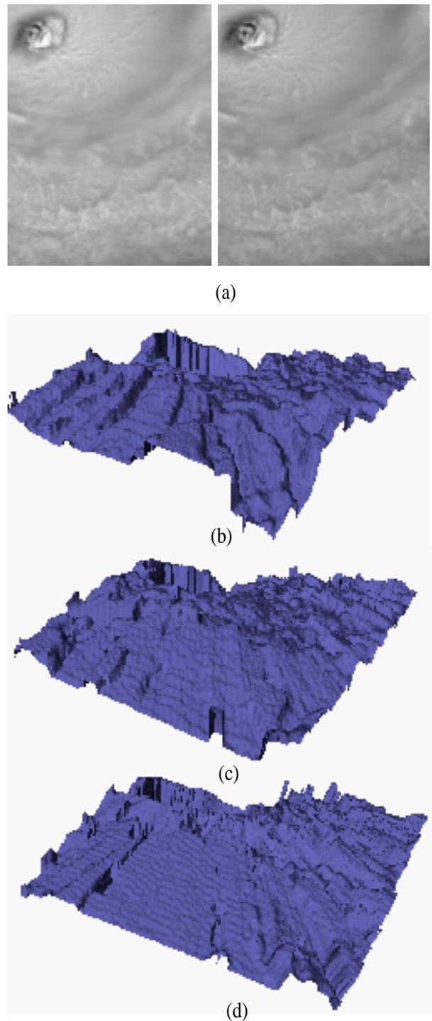
Figure 6: Tracked cloud surfaces. (a) Stereo image pair of the first frame (b) Recovered surface for the first frame (c-d) Tracked surfaces for the second and third frame
