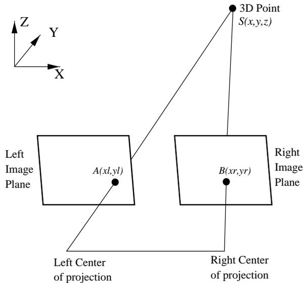
Figure 1: Projection of 3D scene points on the image planes
