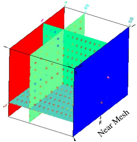
Figure 3: A coarsely initialized 3D array  $V$ . The blue and red planes show the initial positions of near and far mesh, respectively.
