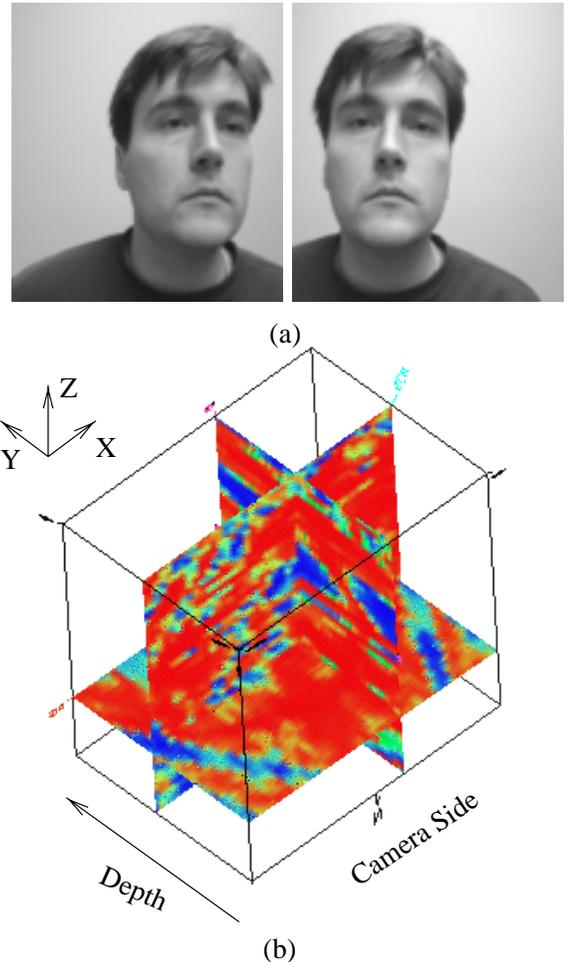
Figure 2: (a) A rectified stereo pair (b) Visualization of the 3D array  $V$  filled by correlation values. Red represents higher correlation values.
