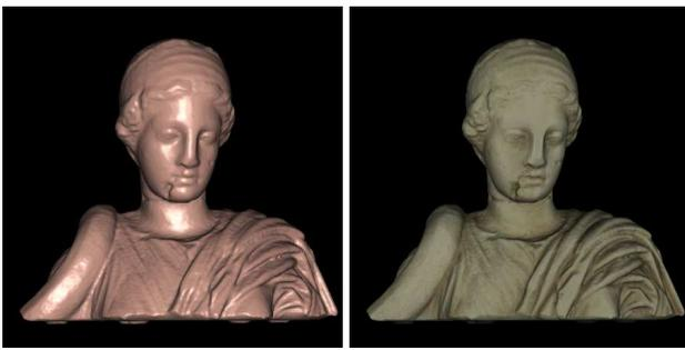
Figure 5. Hygieia model after convergence (159534 vertices). Left: Gouraud shading. Right: texture mapping.
