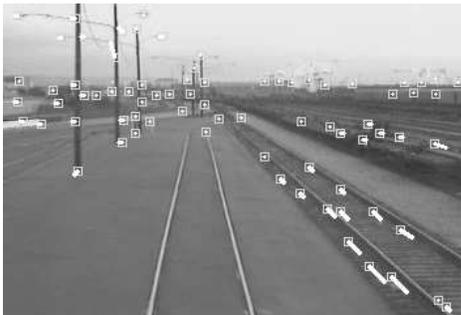
Figure 3. Detected corner features (square boxes) and their optical flows. Note that the line features can cause false matches (aperture problem). The optical flows were exaggerated by 3 times for the visibility.
