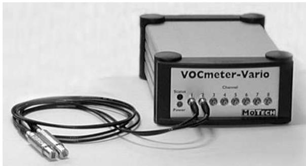
Figure 2: The commercial odour sensing system VOCmeter Vario<sup>4</sup>. The basic unit of the used system can be seen on the right side of the picture. It is able to operate up to eight tube-shaped sensor sticks (like the ones shown in the left side of the picture) over thin coax cables. Notice that the basic unit is placed inside the robots body during the performed investigation (see fig.1).
