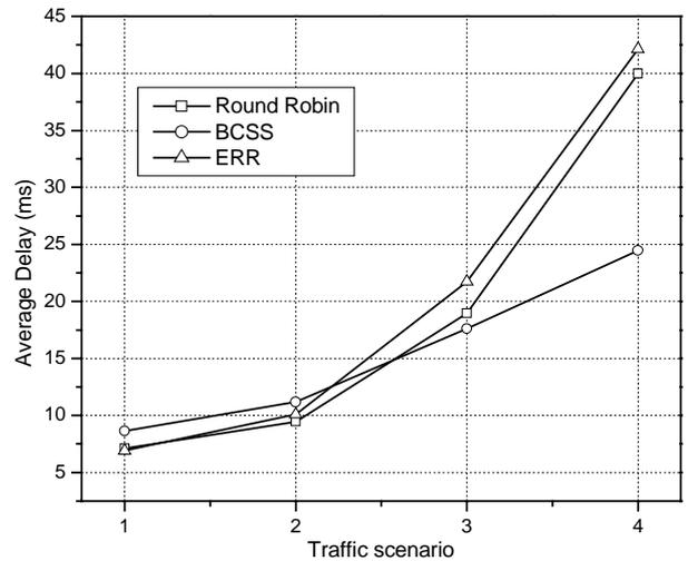
Fig. 4. Average delay for different traffic scenarios
