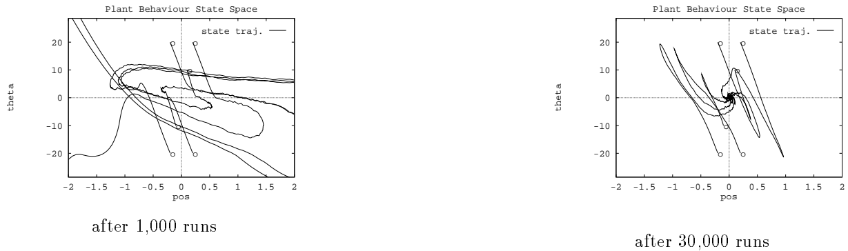
Fig. 3: Evolution of controller capabilities during the learning process for six different starting positions (marked by a circle)
