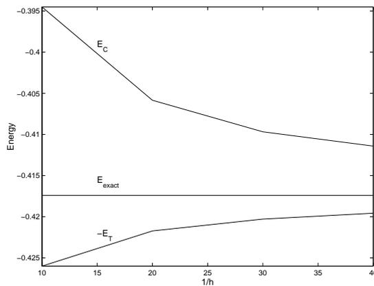
Figure 4. Convergence curves for the crack problem
