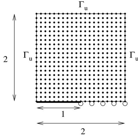
Figure 3. Cracked plate with prescribed displacement on three sides (21 × 21 nodes)
