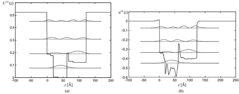
Fig. 1. (a) The stepwise-constant SA-preoptimized, and (b) the variationally fully optimized smooth potential, providing maximal second harmonic generation. Also displayed are the relevant bound state wave functions squared.
