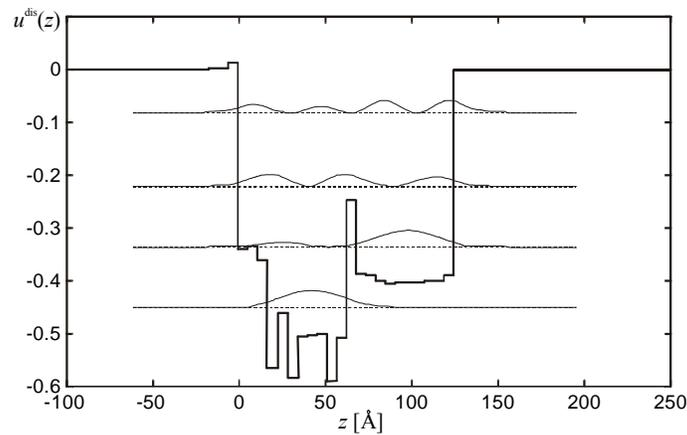
Fig. 2. The discretized, step-graded version of the optimal potential from Fig. 1b, with 2 monolayers wide steps.
