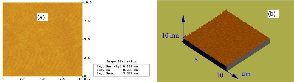
Fig. 3. 2D (a) and 3D (b) AFM surface morphology pictures of an 8  $\mu\text{m}$  thick hybrid sol-gel coating.
