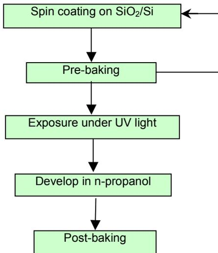
Fig. 1. Flowchart for sol-gel waveguides development.
