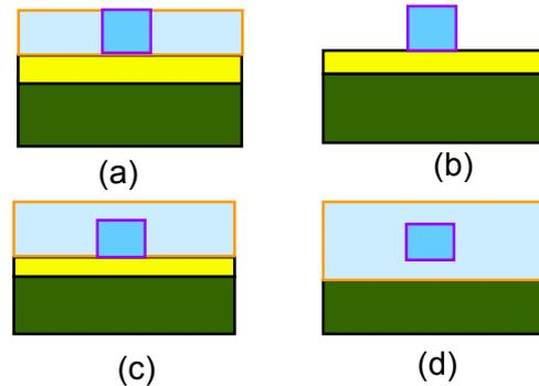
Fig. 2. Different sol-gel waveguides structures. (a), Surface waveguide; (b), Ridge waveguide; (c), Non-symmetry buried waveguide; (d), Symmetry buried waveguide.
