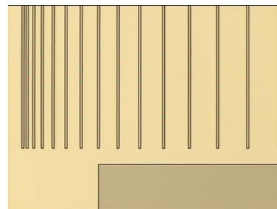
Fig. 4. Optical microscope picture of a series 10  $\mu\text{m}$  strip waveguides with separations from 10 to 200  $\mu\text{m}$ .
