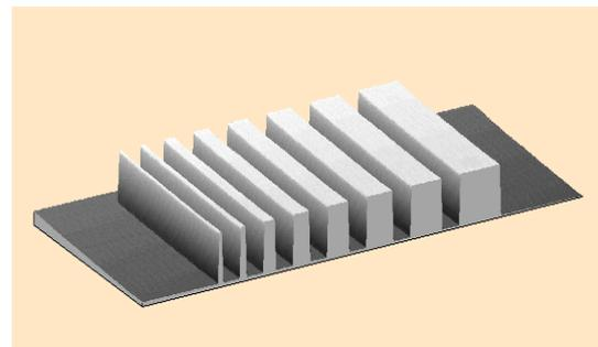
Fig. 5. 3-dimension picture of an 8- $\mu\text{m}$  thick coating with widths ranging from 10 to 200  $\mu\text{m}$ .
