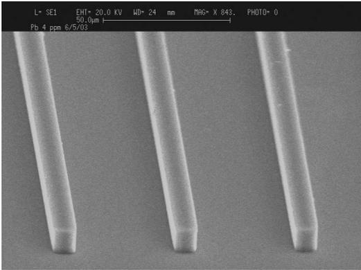
Fig. 6. SEM micrograph of a series of Hybrid sol-gel strip waveguides of 10  $\mu\text{m}$  wide and 8  $\mu\text{m}$  thick.
