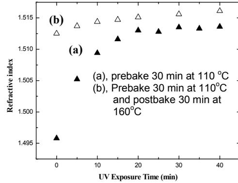
Fig. 7. Refractive index change as a function of UV-exposure time. Samples were prebaked at 110°C for 30 min (a) and further post-baked at 160°C for 30 min (b).
