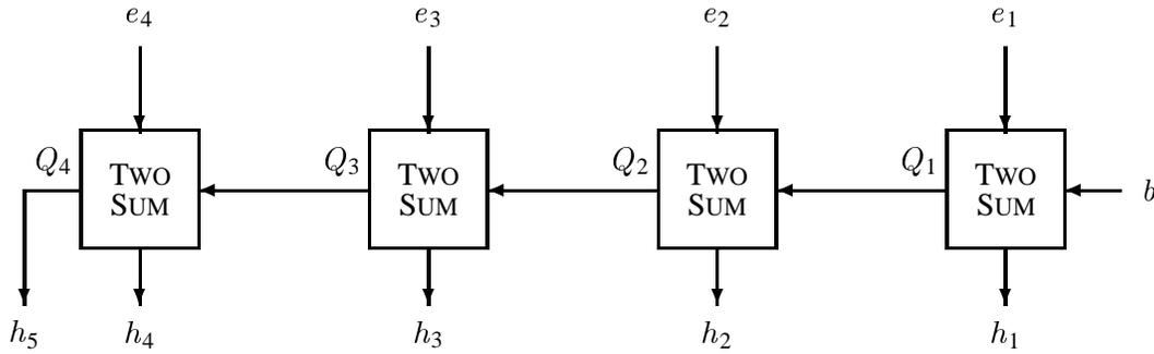
Figure 6: Operation of GROW-EXPANSION. The expansions  $e$  and  $h$  are illustrated with their most significant components on the left. All TWO-SUM boxes in this report observe the convention that the larger output ( $x$ ) emerges from the left side of each box, and the smaller output ( $y$ ) from the bottom or right. Each  $Q_i$  term is an approximate running total.
