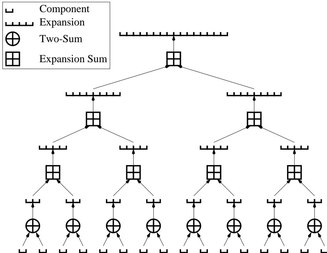
Figure 16: Distillation of sixteen  $p$ -bit floating-point values.
