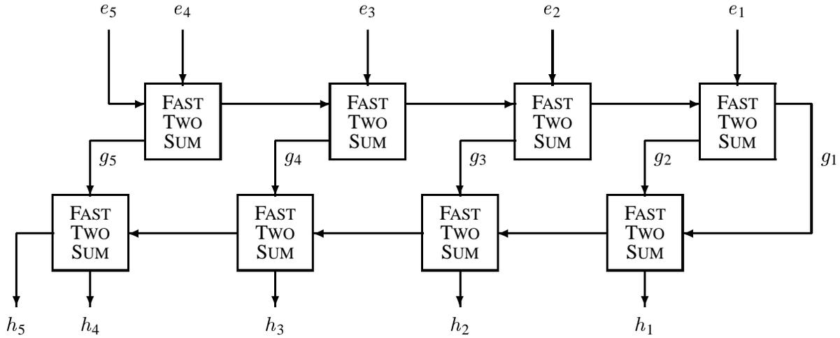
Figure 15: Operation of COMPRESS when no zero-elimination occurs.
