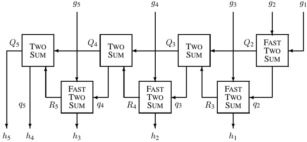
Figure 23: Operation of LINEAR-EXPANSION-SUM.  $Q_i + q_i$  maintains an approximate running total. The FAST-TWO-SUM operations in the bottom row exist to clip a high-order bit off each  $q_i$  term, if necessary, before outputting it.
