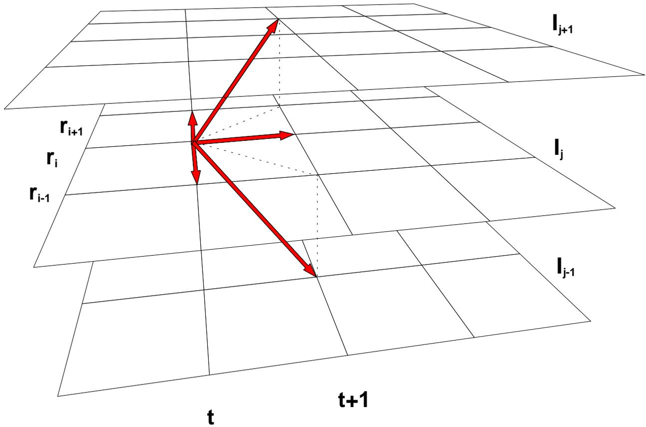
Figure 3: Extended Crank Nicholson algorithm.
