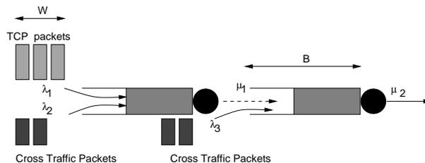
**Figure 2.** Arrival of TCP packets at Bottleneck
