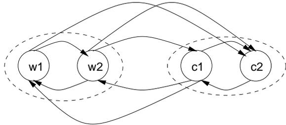
Figure 5. Hidden Markov Model with hidden delay dimension
