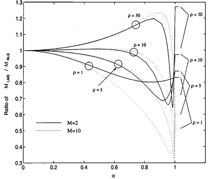
Fig. 4. Ratio of the LMS excess misadjustment vs. RLS excess misadjustment.
