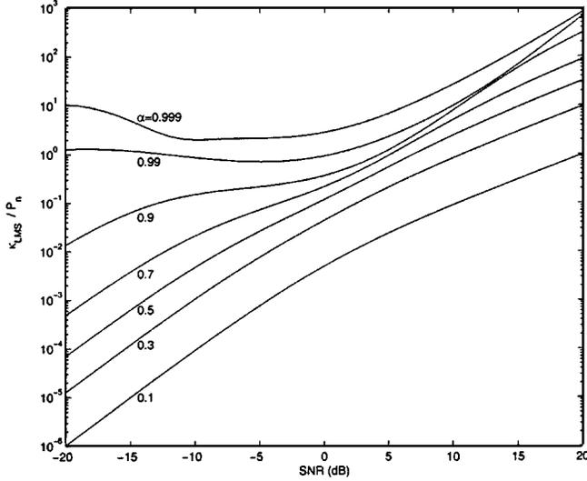
Fig. 3. Normalized asymptotic lag misadjustment  $\lim_{M \rightarrow \infty} \kappa_{LMS}/P_n$  versus SNR for a chirped AR1 signal with correlation  $\alpha$  embedded in white noise. Results are shown for  $\alpha$  between 0.1 and 0.99.
