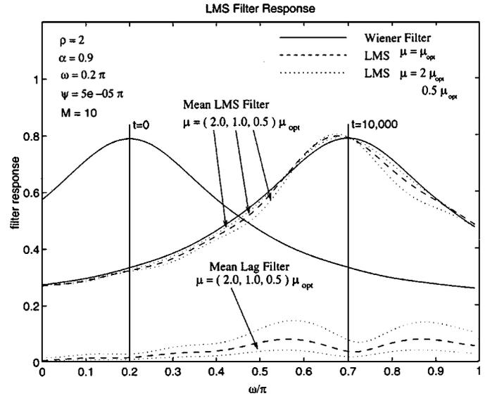
Fig. 1. LMS filter transfer function over time for a chirped AR1 process.
