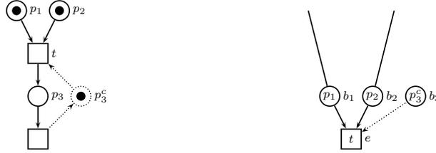
Figure 5. Parts of a 1-safe Petri net and its unfolding
