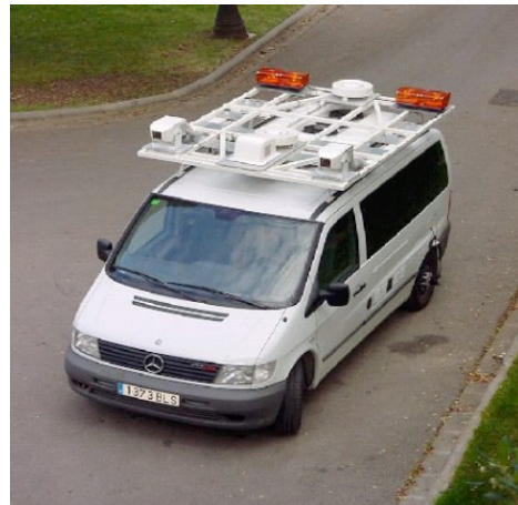
Figure 1: Geomòbil system developed at ICC
