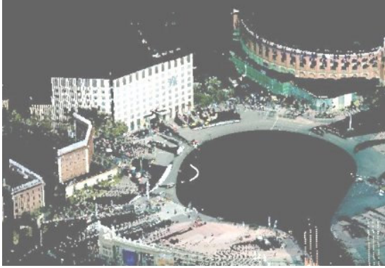
Figure 8: RGB laser points collected in a kinematic survey (laser looking to the right side of the van)
