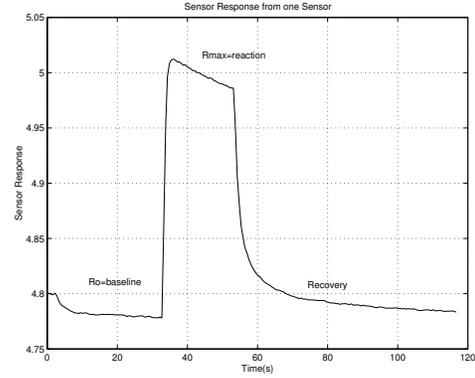
**Figure 1.** Example of sensor data throughout the three phases of sampling an odour with one of the 32 gas sensors.
