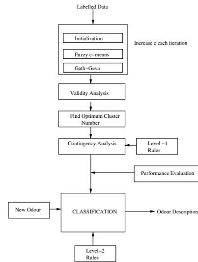
**Figure 2.** Overview of the system that forms odour categories using electronic nose data
