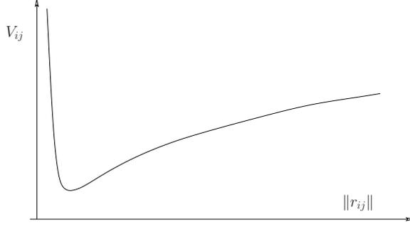
Fig. 2. Example of inter-agent artificial potential function.
