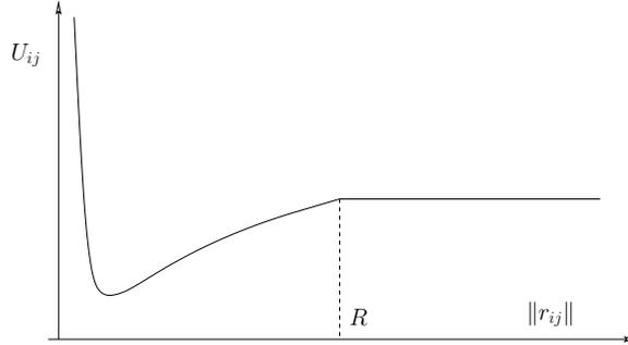
Fig. 3. A saturated nonsmooth artificial potential function.
