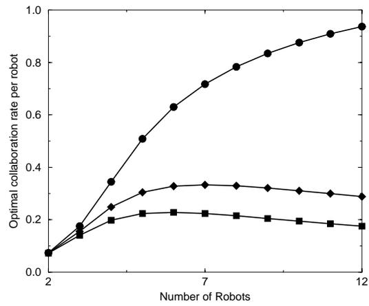
Figure 9: Relative collaboration rate vs the number of robots for different values of interference strength:  $\tau_{av} = 0$  (circles),  $\tau_{av} = 0.5$  (diamonds) and  $\tau_{av} = 1.0$  (squares).
