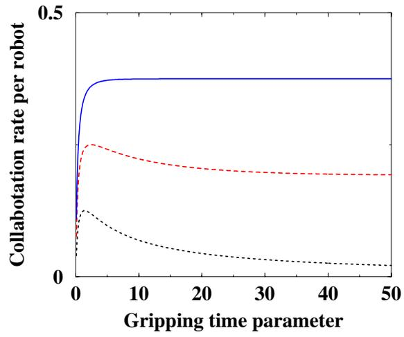
Figure 8: Collaboration rate per robot vs (dimensionless) gripping time parameter  $\tau$  for  $\beta = 0.5$  (short dash),  $\beta = 1$  (long dash),  $\beta = 1.5$  (solid line). These values of  $\beta$  correspond, respectively, to two, four, and six robots in the experiments with four sticks (*cf.* Fig. 5).
