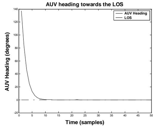
Fig. 6. AUV heading towards and tracking the LOS
