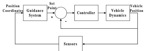
Fig. 1. Navigation, guidance and control of a vehicle
