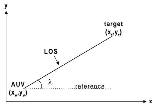
Fig. 5. AUV-target engagement geometry
