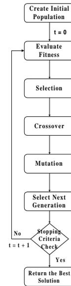
Fig. 4. Flowchart of a simple genetic algorithm
