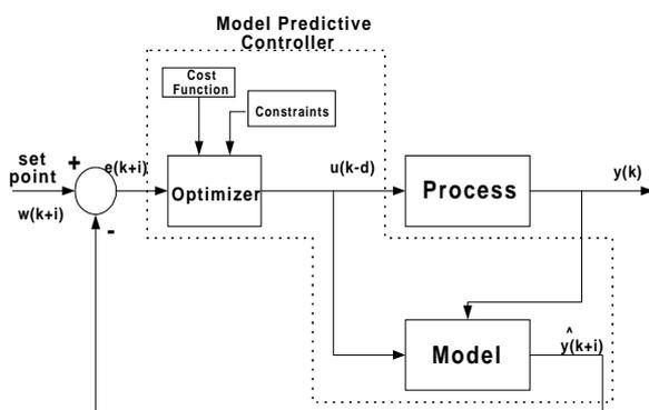
Fig. 2. Structure of Model Predictive Control
