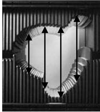
Figure 2: Multileaf collimators with movement of leaves indicated.
