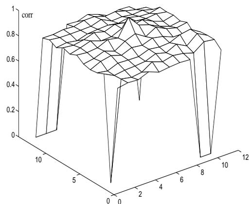
**Figure 3.3** Sensitivity to translation when a correlation threshold of 0.7 was used together with a hit threshold of 20%. A strong match is supported even when the robot is moved 50 cm in either direction away from the learned template position. (The axes indicates the different samples.)
