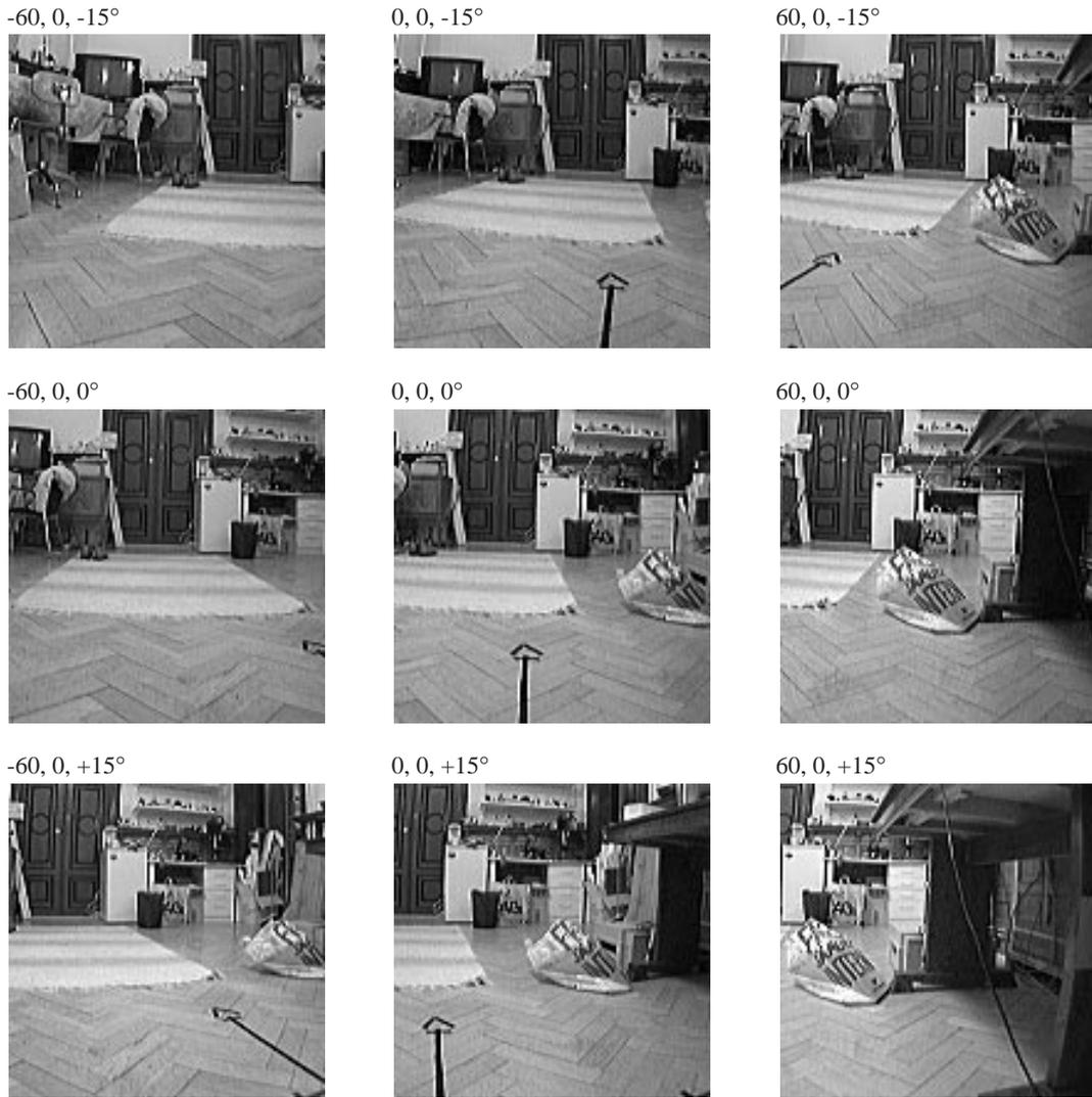
**Figure 3.5.** Rotations sensitivity within a view-field. The coordinates indicate the distance from the central position and the angle away from the forward direction of the view-field.
