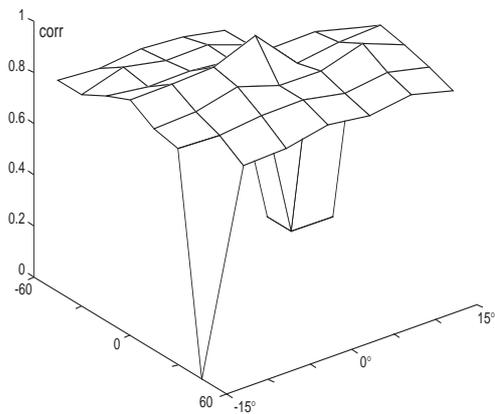
**Figure 3.5.** Sensitivity to translation combined with rotation of the robot. The template matches the input image as long as the angle is less than  $15^\circ$  or the robot is less than 60 cm from the learned location. Parameters were set as in figure 3.3.
