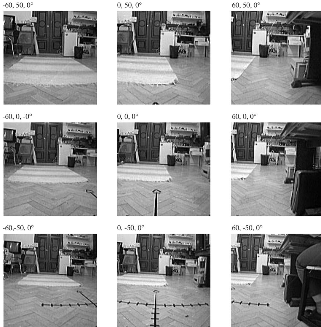
**Figure 3.1.** Translation sensitivity within a view-field. The figure consists of nine views within a single view-field with a size of approximately  $1\text{m}^2$ . The coordinates indicate distance in cm from the central position. The central image shows the position where the template was learned.
