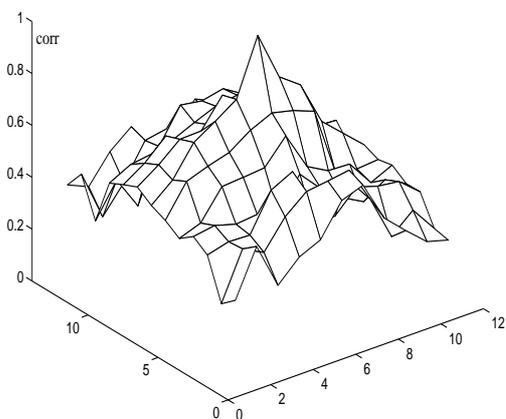
**Figure 3.2** Sensitivity to translation when all feature are allowed to contribute to the average correlation. The match level decreases smoothly as the robot is moved away from the location where the template was learned. (The axes indicates the coordinates of the different samples.)
