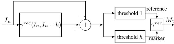
Figure 5. Block diagram of the high contrasted areas detector ( $\gamma^{rec}$  is the morphological reconstruction).
