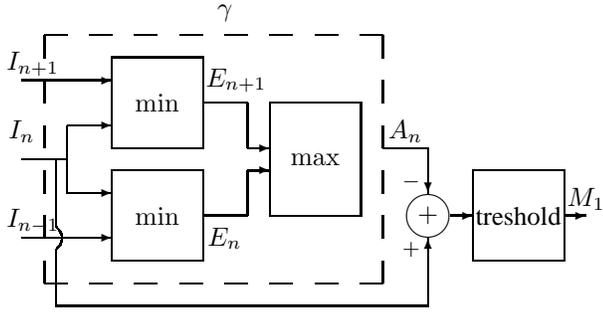
Figure 3. Block diagram of the Temporal Opening method.
