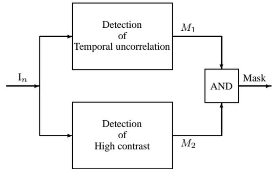
Figure 2. Block diagram of the blotch detection process.
