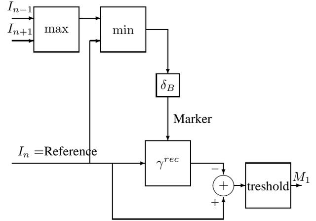
Figure 4. Block diagram of the Opening by Reconstruction method using marker dilation.  $\gamma^{rec}$  is the morphological reconstruction and  $\delta_B$  the morphological dilation.
