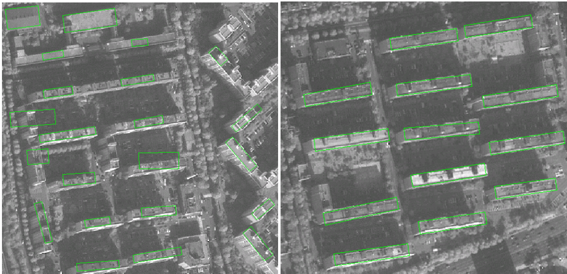
Figure 12. Results of building extraction. The left image is the results of building rectangle estimation line analysis and template matching only (without manual editing). The right image is the results of building template matching.
