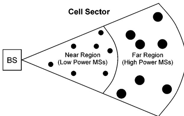
Fig. 1. User location and transmit power distribution model for simple two-region BS.  $N_{near}$  and  $N_{far}$  are the numbers of low and high power MSs in the “near” and “far” regions, respectively.
