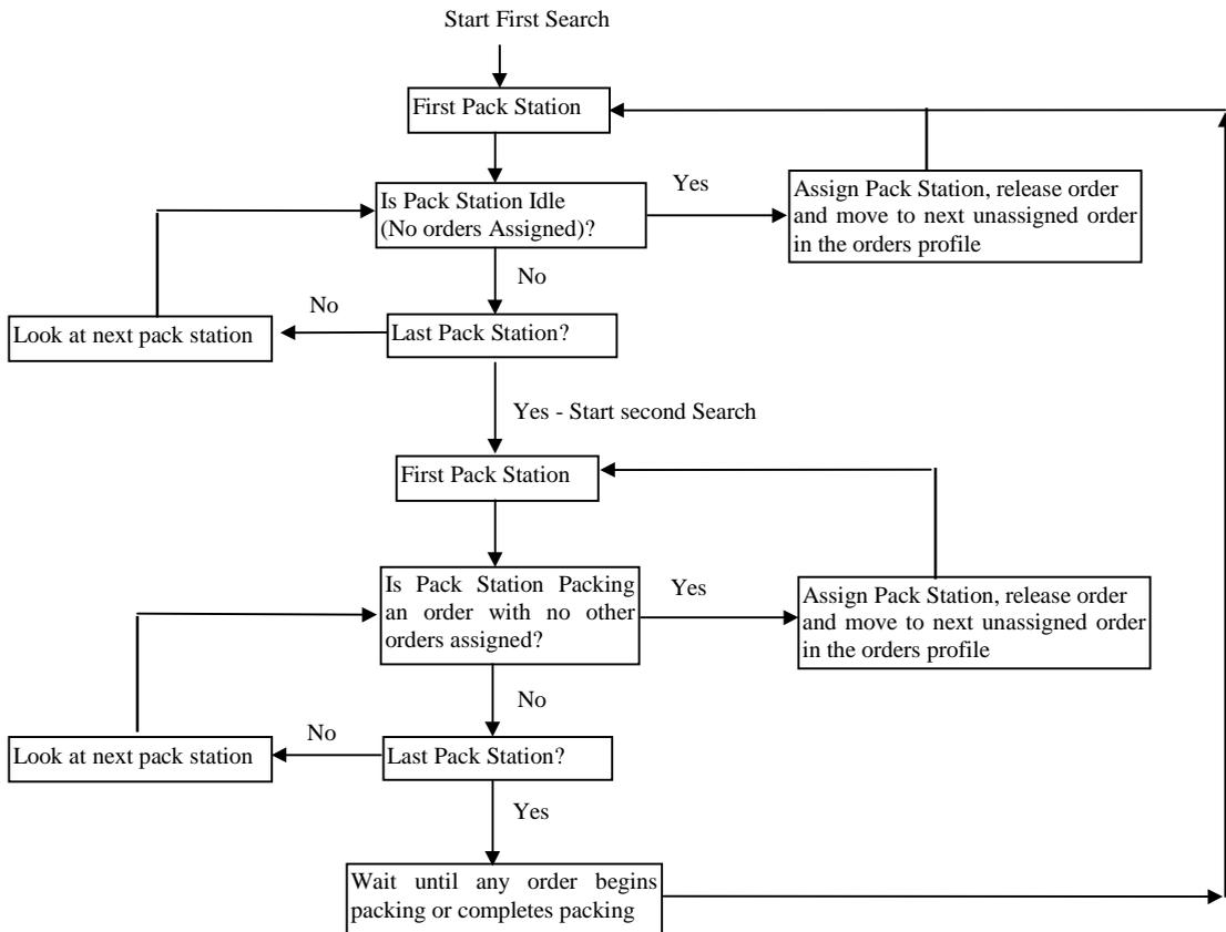
Figure 3: FIFO Pack Station Assignment Algorithm
