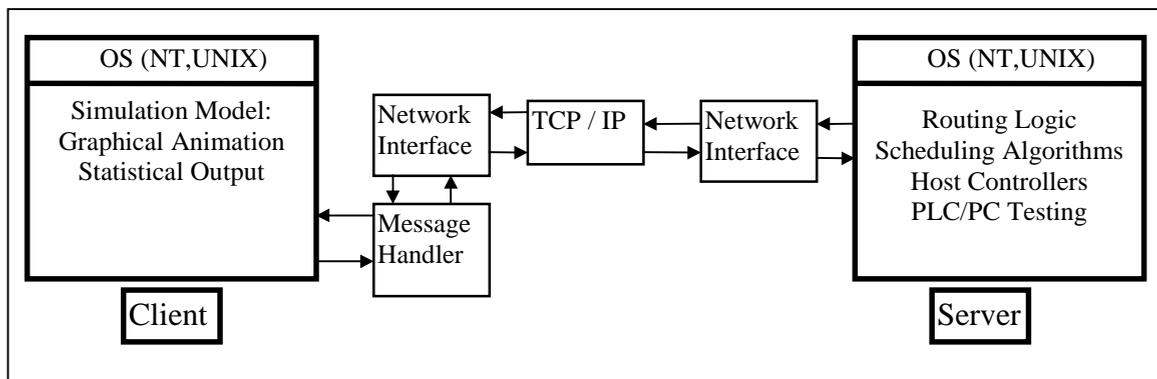
Figure 2: Typical Emulation Structure
