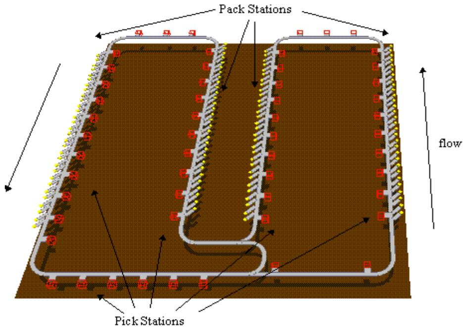
Figure 1: A Pick and Pack Conveyor System
