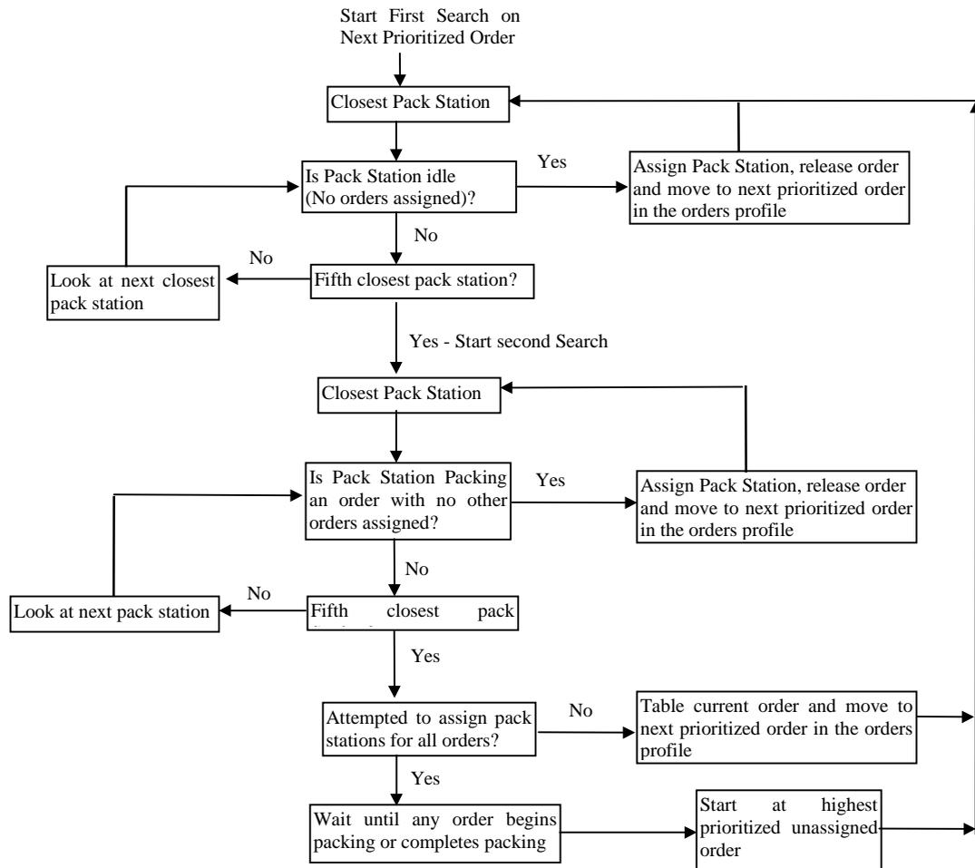
Figure 4: RULE1 Pack Station Assignment Algorithm
