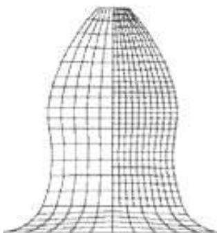
Figure 6: Front view of the tooth where fine and thick mesh are appreciated.
