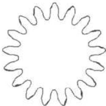
Figure 1: Profile of spur gear showing the wear of teeth.
