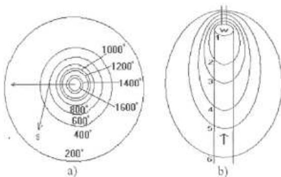
Figure 3: Isotherms caused by (a) immobile source and (b) mobile source.
