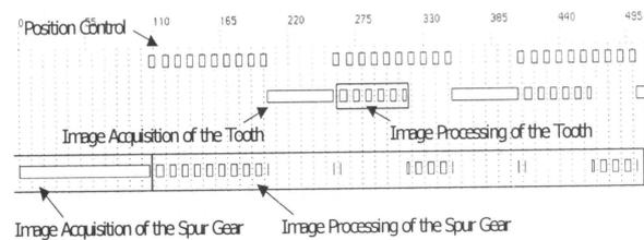
Figure 9: Chronogram showing the execution time of the tasks in the Mode 2
