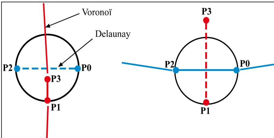
**Figure 6** The Delaunay edge P0-P2 has no circle empty of Voronoi vertices in the example on the left - hence its dual P1-P3 is part of the skeleton. On the right the empty circle indicates that the Delaunay edge is part of the crust.
