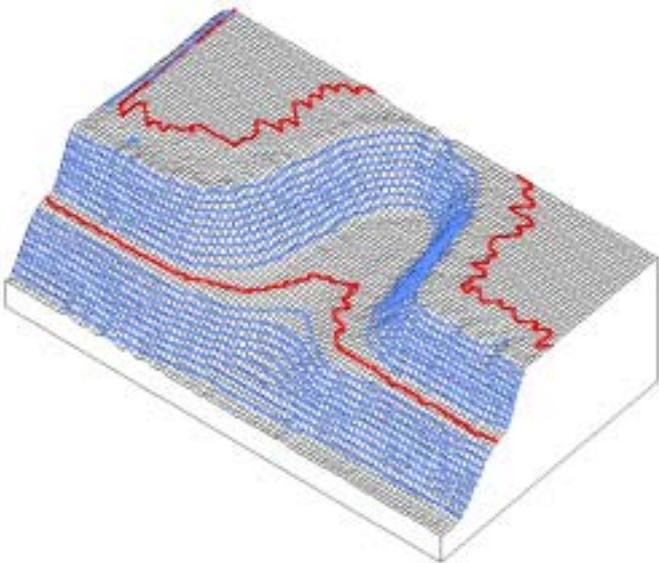
Figure 28 Inverse-distance grid interpolation for the data of Figure 27
