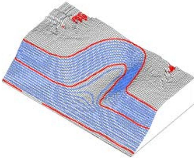
**Figure 29** Simple kriging grid interpolation for the data of Figure 27
