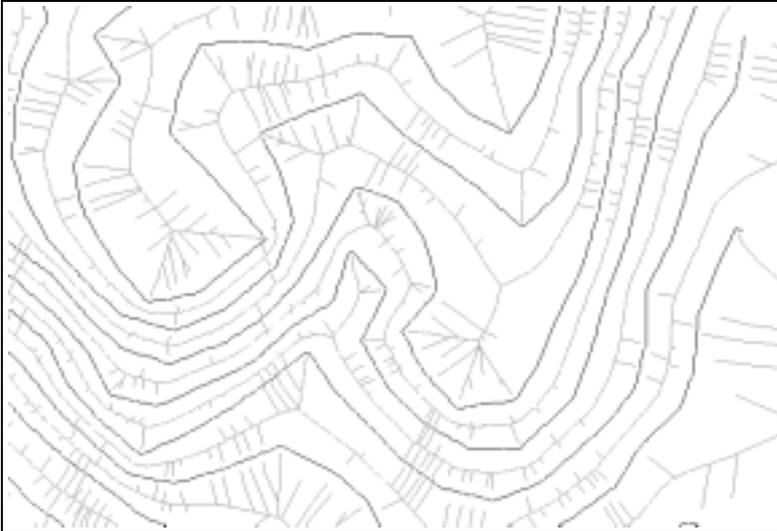
**Figure 11 Crust and skeleton of a simple contour map**
