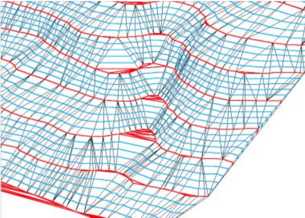
**Figure 20** Contours interpolated from the triangulation of **Figure 19**
