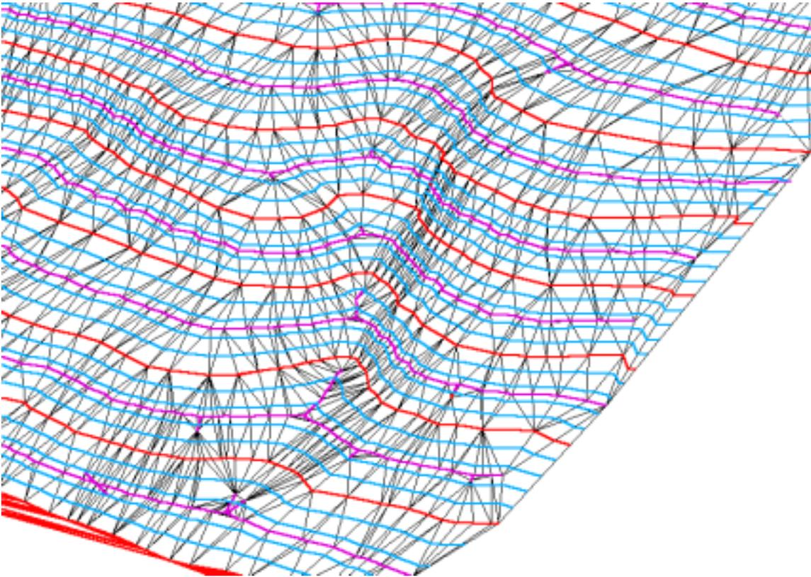
**Figure 22** Contours interpolated from the triangulation of Figure 21
