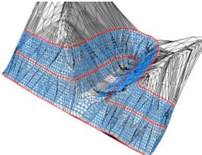
**Figure 30** Area-stealing interpolation for the enriched data of Figure 27
