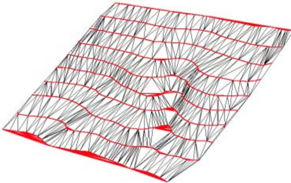
**Figure 19 Perspective view of a simple triangulation of contour data**
