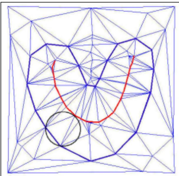
**Figure 5** Amenta et al.'s construction for crust extraction
