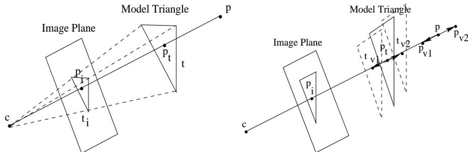
Figure 2: One dimensional visibility test. (a) Model's triangles and features are tested for 2D overlap in the image plane. (b) Representation of 1D variance of  $\mathbf{p}, \mathbf{p}_t$  along the projection optical ray.
