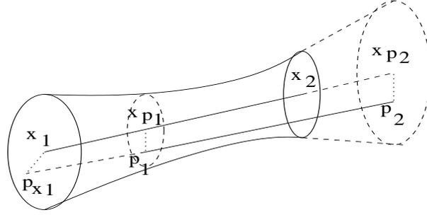
Figure 1: Feature update process. New line measurement  $\mathbf{x}$  checked for consistency and combined with corresponding model line  $\mathbf{p}$
