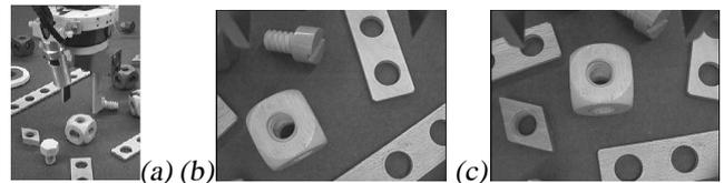
**Figure 1. The end-effector over the target: (a) the gripper and the hand camera. A “cube” viewed by the hand camera before (b) – and after the fine positioning (c). Note the tool tips in the upper rim of (b,c).**
