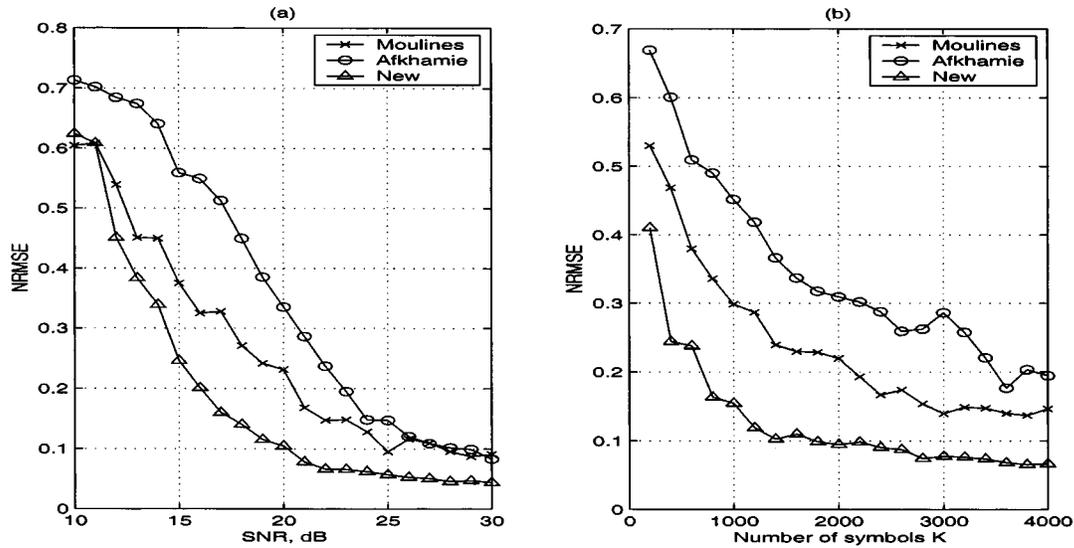
Fig. 3. NRMSE of the estimated channel response using  $m = 6$  versus (a) SNR using  $K = 2000$  data samples. (b) Number of samples  $K$  for SNR = 20 dB (averaged over 100 runs).
