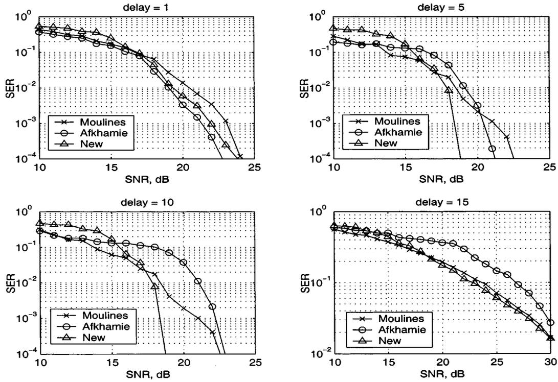
Fig. 5. SER obtained by the length  $m = 12$  MMSE equalizers (averaged over 100 independent runs).
