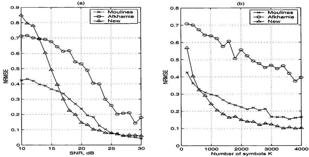
Fig. 6. NRMSE of the estimated channel response using  $m = 12$  versus (a) SNR using  $K = 2000$  data samples. (b) Number of samples  $K$ , for SNR = 20 dB (averaged over 100 runs).
