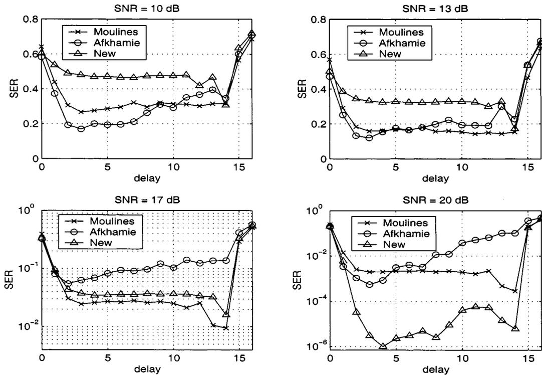
Fig. 4. SER obtained by the length  $m = 12$  MMSE equalizers (averaged over 100 independent runs).
