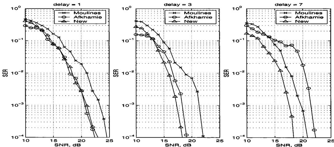
Fig. 2. SER obtained by the length  $m = 6$  MMSE equalizers (averaged over 100 independent runs).
