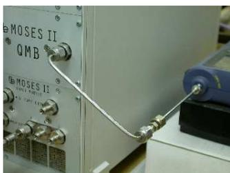
Figure 1: The connection between MOSESII and Cyranose 320. The out-pipe of the *QMB* module is connected to the 2" needle at the sample inlet of Cyranose 320. This connection is mediated by a tailor made non-sealing adapter, which directs part of the sample into Cyranose 320, and allows the rest to evaporate in the room.
