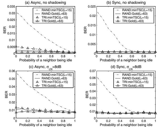
Fig. 9. Comparison of link-level BER performance of the random and triangular topology when using MMSE receivers.
