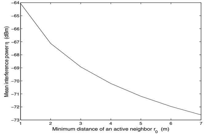
Fig. 4. Mean interference power from a neighboring transmitter (eq.(9)). As in Fig. 3,  $r_R = 25$  m,  $r_I = 56$  m,  $n = 3.0$ , and  $P_r = -70$  dBm.
